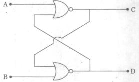
In the above circuit, if the inputs A = B = 0, then what are the possible logic states of C and D respectively?
