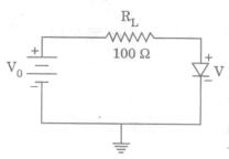
In the above circuit  $V_0 = 2$  volt, V = 2 volt. What is the current flowing through the diode?
