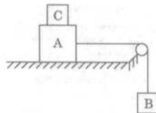
In the above figure, block A is 4.4 kg and block B is 2.6 kg in mass. The coefficient of static friction between A and the horizontal surface is 0.20. What is the minimum mass of C to prevent horizontal sliding ?
