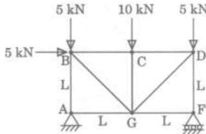
In the pin-jointed truss as shown above, the horizontal deflection of roller support will be the sum of deformations in members
