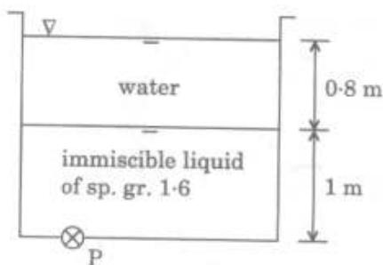
What is the gauge pressure at point P in the figure ? Assume  $g = 10 \text{ m/s/s}$ .
