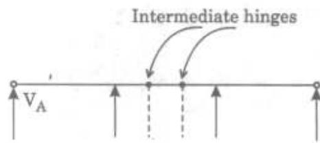
For a balanced cantilever bridge, which one of the following corresponds to the influence line diagram for the left end reaction  $V_A$  ?
