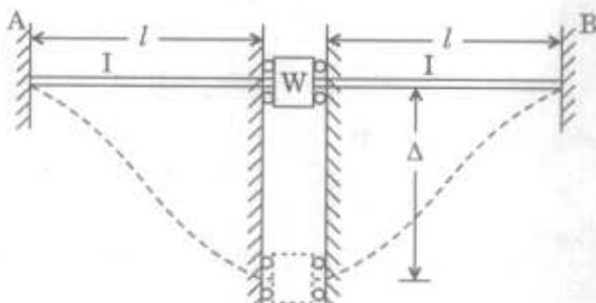
A heavy weight attached to a rod can slide in a grooved support as shown. What is the equilibrium sliding distance  $\Delta$  ?
