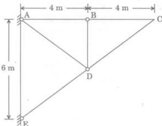
If the member CD has been fabricated 10 mm short, by how much will point C deflect vertically in mm?
