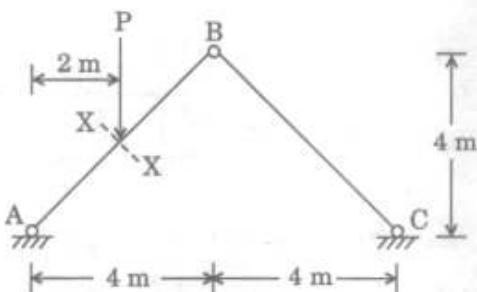
What is the shear force at section XX in the free-hinged frame in the above figure ?
